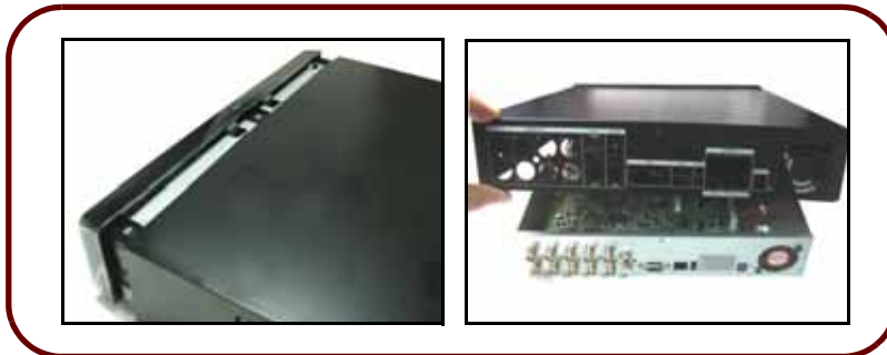
Figure 44.0 Slide the cover and lift away from housing
